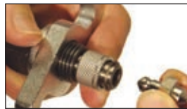
Quick Chuck for Fast Punch Changeover
