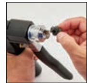
Detent ball provides quick punch change
