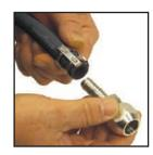
Place clamp onto hose, push adapter into hose.
