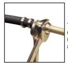
Tighten compression union onto aluminum line.
