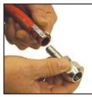
Place clamp onto hose, push adapter into hose.
