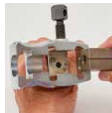
Magnetic yoke holds dies securely in place
