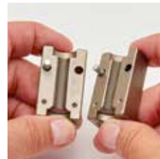
Pins ensure accurate alignment of dies
