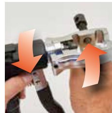
Two-piece design allows for swivel action
