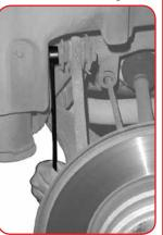
\*61600 FAN CLUTCH WRENCH U.S. PATENT 6,912,936 Universal fan clutch wrench works with all "BOLT ON" water pumps that have bolts holding the pulley on the pump. 95260 40mm use with 61600 for 1992-1996 Econoline Vans, 1993-1996 F Series Pickup trucks, with 4.9L engines.
