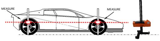
At the center point of the front wheel of the vehicle measure the distance from the floor to the point where the laser strikes the tape measure, RECORD.
