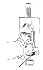
The leg design allows you to push on the driveline or on the U-Joint cross. (Works either way on virtually all class 7 or 8 U-Joints).
