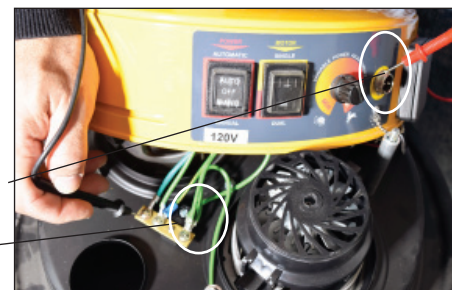
Connector for Pressure Switch Lead Grounding Bus
