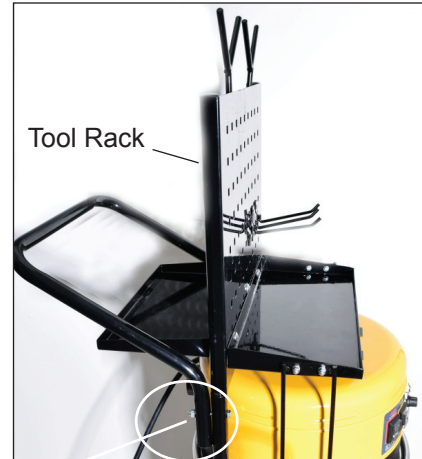
Remove bolt that secures the handle, upright and frame.
