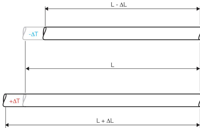
The prevention of such a variation in length in the material would generate a tensile stress (with  $\Delta T < 0$ ) or a compression stress (with  $\Delta T > 0$ ) given by:
