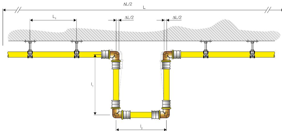
The total length of the “omega” expansion bend  $L_B$  [mm] is calculated using the formula (also shown in the following diagram):
