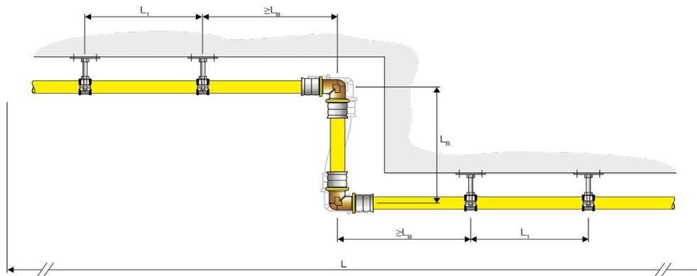
The length of the flexible arm  $L_B$  [mm] is calculated using the formula:
