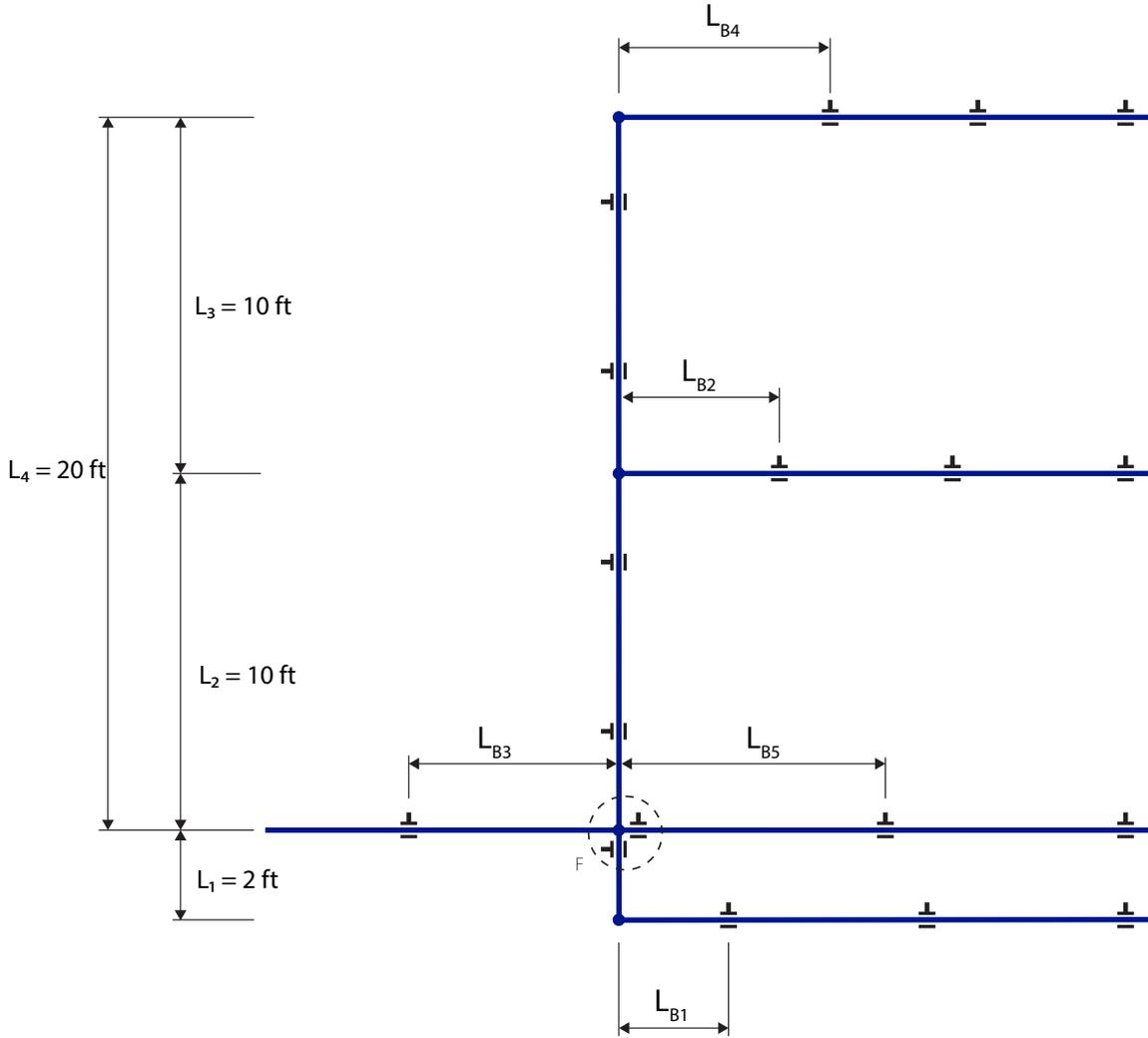
The pipe sections  $L_{B3}$  and  $L_{B5}$  are not subject to flexure due to the anchor point (F) near the cross branch. The sections subject to flexure are:
