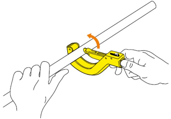
2. Calibrate and chamfer the pipe to obtain a perfectly round inner circumference of the pipe. Always make sure that the reamer has no dents or damage as they would damage the pipe and compromise the seal.
