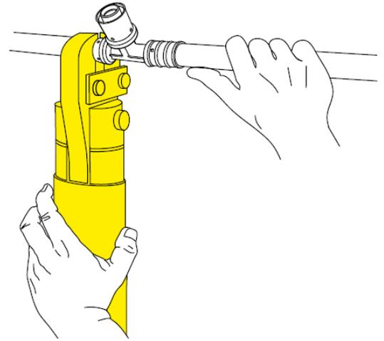
For manual crimper: position the manual crimper so that the crimping jaw is aligned and in position with the respect of the body of the fitting and close the tool completely until it clicks (for more details refer to the instructions supplied with the tool).
