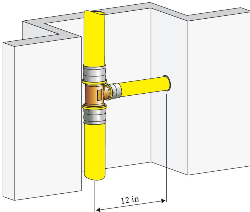
From the figure we can see that the available space for creating a flexible arm is  $L=12$  in, which is the distance between the wall, through which the change in direction passes, and the riser.
