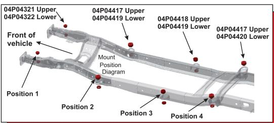
To remove the metal inside the lower mounts, use a razor knife and pie cut the O.E. rubber .
