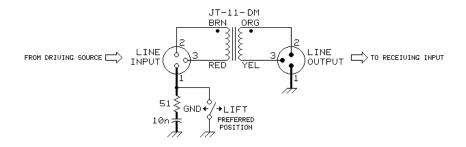
AN OUTPUT TRANSFORMER BOX CAN BE VERY USEFUL TO REDUCE OR ELIMINATE "HUM" IN AUDIO SYSTEMS. IT WILL USUALLY DO A GOOD JOB AT ELIMINATING "HUM", BUT IS MUCH LESS EFFECTIVE AT THE HIGHER FREQUENCIES CONTAINED IN "BUZZ". IT WILL ALSO ALLOW AN "ACTIVE BALANCED" OUTPUT TO DRIVE GROUNDED (UNBALANCED) LOADS. AN INPUT TRANSFORMER, INSTALLED AT THE CABLE'S RECEIVE END, IS THE BEST SOLUTION FOR BOTH "HUM" AND "BUZZ". <SEE JENSEN AN003 FOR MORE DETAILED INFORMATION>
