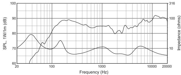
Frequency Response, on axis in half-space ( $2\pi$ , flush mounted in ceiling) Thru (8  $\Omega$ ), with Input Impedance
