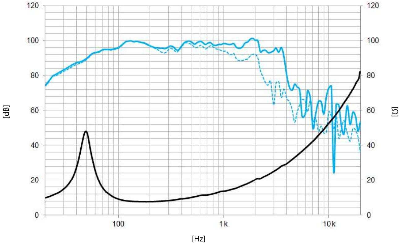
Note: Frequency response measured with loudspeaker standing on infinite baffle in anechoic chamber, 1W @ 1m
