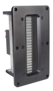
Impedance: 8ohms Rated Power: 100W Sensitivity: 102dB/W/m Frequency range: 900Hz-40kHz Dimension of ribbon(mm): 14.5W×150L×0.01T Shape of ribbon: wave Mass of ribbon: 51mg Moving area of ribbon: 2175 square millimeter Gap flux: 0.36Tesia Recommended crossover frequency: 2000Hz Material of faceplate: aluminum Dimension of faceplate(mm): 106W×190H×6T Outside dimension(mm): 106W×190H×110D Net weight: 3.8kg/pc
