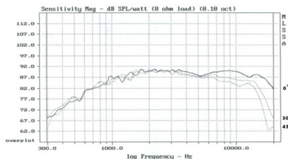
Measured on IEC baffle using Brüel & Kjaer 3144 model microphone.
