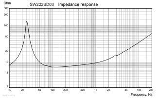
Measuring conditions, impedance Driver mounting: Free air, no baffle, back side open (no cabinet) Input signal: Stepped sine wave, semicurrent-drive, nominal current 2 mA Smoothing: None
