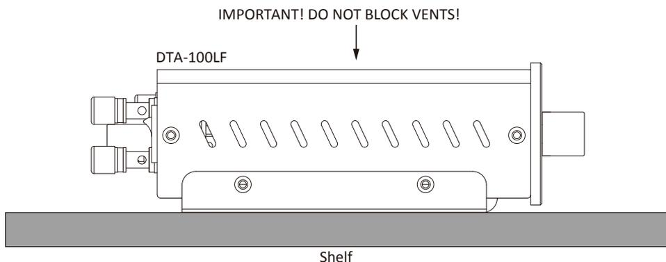
Do not block the side vents. Even though the DTA-100LF will typically run cool, the side vents allow air to circulate through the chassis. Do not block the vents for any reason.
