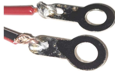
Wires soldered to terminals
