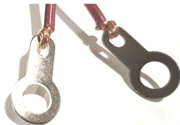
Wire wrapped through terminals
