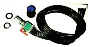
16. Locate the On-Off Switch And Cable and DC Input And Cable. Remove the nut and lock washer from the DC input and install the jack in the corresponding hole in the panel. Add the lock washer then nut and tighten nut using the supplied wrench. Install the On-Off switch through the front of the panel and press until it snaps into place.
