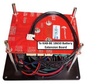
22. Install the KAB-BE 18650 Battery Extension Board to the four 22mm Silver Standoffs with the four Silver M3 x 6 mm Cap Head Screws from the KAB-PMV3 Panel Mount Kit hardware. Tighten screws with the included Hex (Allen) Wrench.
