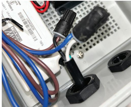
11. Install the outdoor speaker wire (sold separately) through the P9 glands and wire them to the amp following Left/Right and plus/minus silk screen. See wiring diagram below. Once they're installed tighten the gland nuts so the wires don't pull out easily which also prevents moisture from entering the box. Tuck in the AC wires to the left of the power supply away from the amp.
