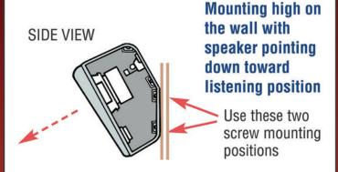
Use template to locate these two screw mounting
