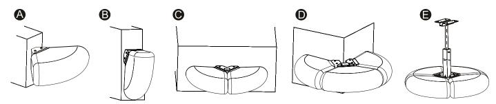
To mark the proper locations for drilling, place the multi-angle bracket against the mounting surface and choose the holes you want to use for mounting. Then use a pencil to mark the hole locations on the mounting surface prior to drilling. Remove the bracket before drilling the holes, in order to avoid damage to the bracket. After drilling the mounting holes, install the large half of the bracket firmly to the mounting surface in the desired orientation using appropriate mounting hardware.
