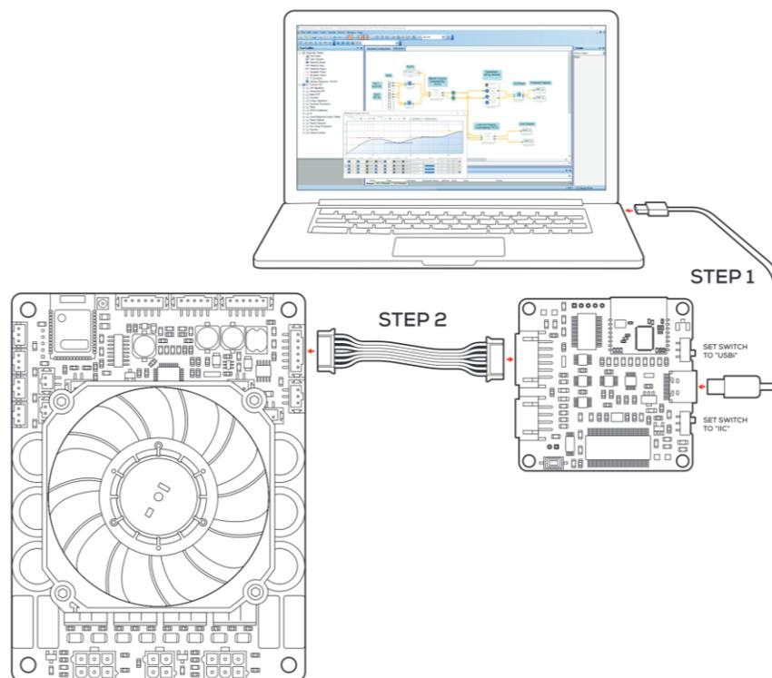
*Pictured is a KABD-4100 amplifier connected to the KPX, which is connected to a Windows Laptop running the SigmaStudio software.*
