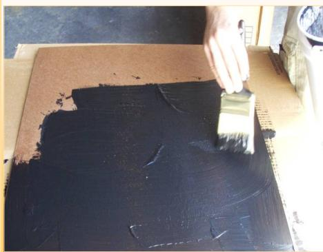
For a demonstration, we simply applied DuraTex (you can use the Spray Grade, Roller Grade or High Build) with a brush to completely cover the substrate... in this case it was simple piece of 1/4" hardboard, but it works on MDF or Birch Ply too.
