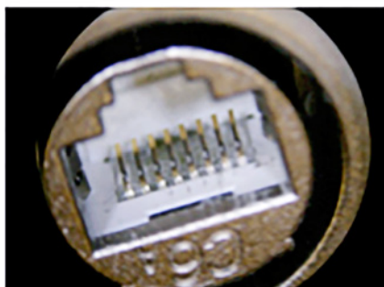
figure 14 – NE8FDX-Y6 after 1000 mating cycles
