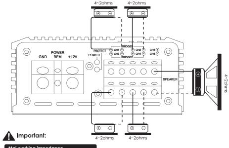
Mai working impedance CH1/4: 2ohm stereo or 4ohm bridged. CH5: 2ohm mono
