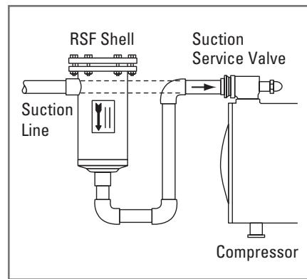
Any pressure loss in the suction line also reduces system capacity significantly. When an RSF shell or replaceable core type Catch-All is used, it is recommended that the cores be removed and filter elements installed when the clean-up job is complete. Obtaining a low pressure drop is particularly important for energy savings on supermarket refrigeration systems. Therefore, suction line filter-driers should be sized generously on these systems.
