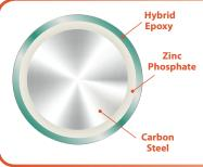
**Proform** - is an economical solution for high humidity or wet applications. The carbon steel is treated with a zinc phosphate base. A hybrid epoxy with an antibacterial agent is electrostatically applied over the treated surface. 15 year limited warranty for antimicrobial finish to not rust or corrode.
