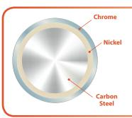
**Chrome** - is a plating process which deposits hard chrome over a cooper, nickel surface. This process is very durable and is used in storage or material handling applications in any dry storage environment. 1 year limited warranty to not rust or corrode when used in dry and non-humid environments.
