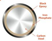
**Black** - treated with an iron phosphate and the powder coated black epoxy is electrostatically applied, baked and cured to a hard surface. 10 year limited warranty for finish to not rust or corrode.
