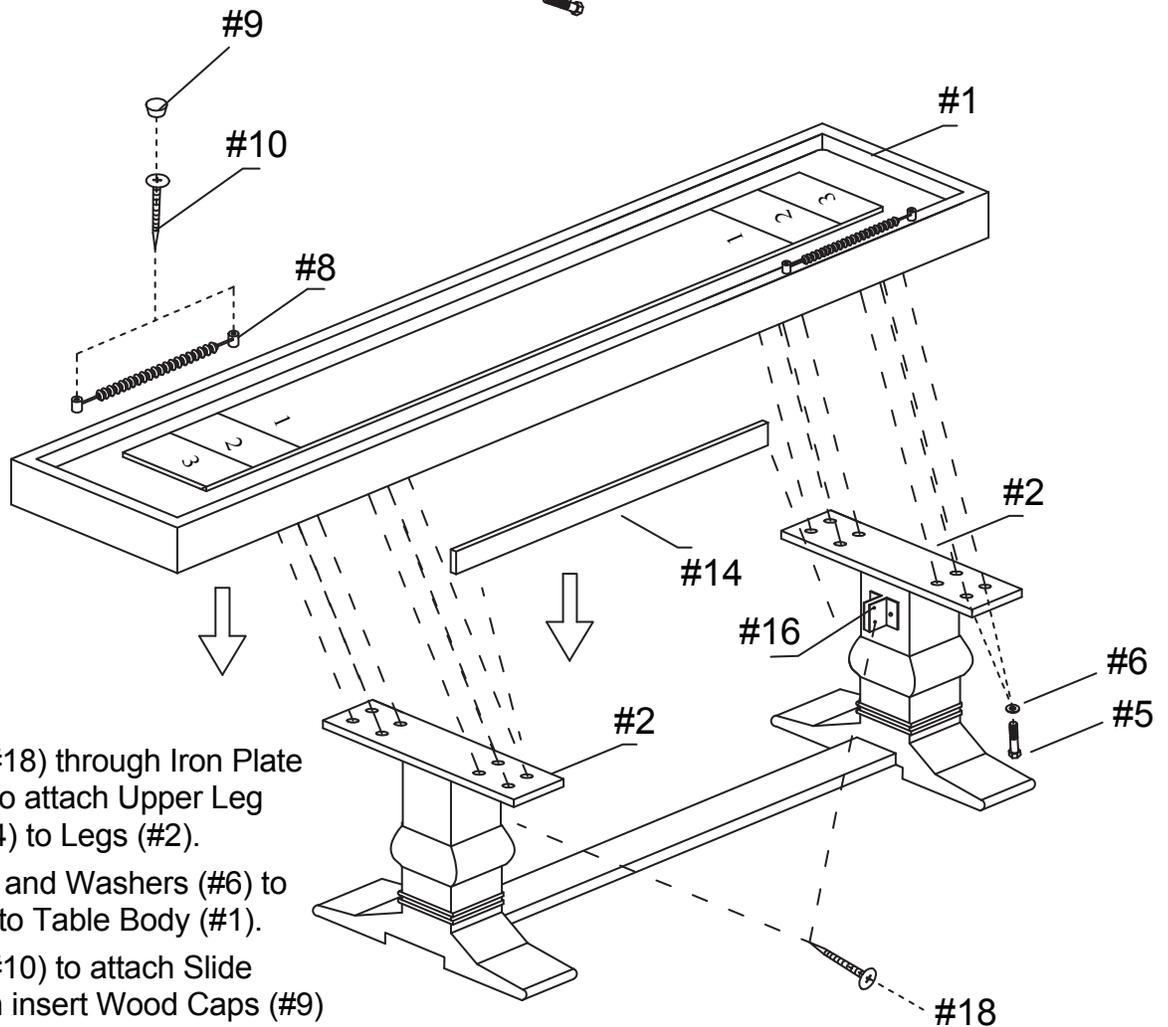
1. Use Screws (#18) through Iron Plate Connector (#16) to attach Upper Leg Cross Brace (#14) to Legs (#2).
