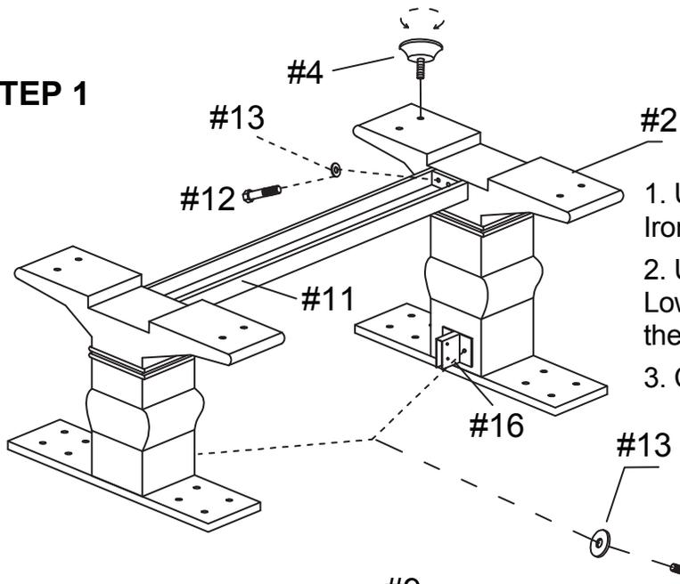
1. Use Bolts (#17) and Washers (#13) to attach Iron Plate Connectors (#16) to Legs (#2).
