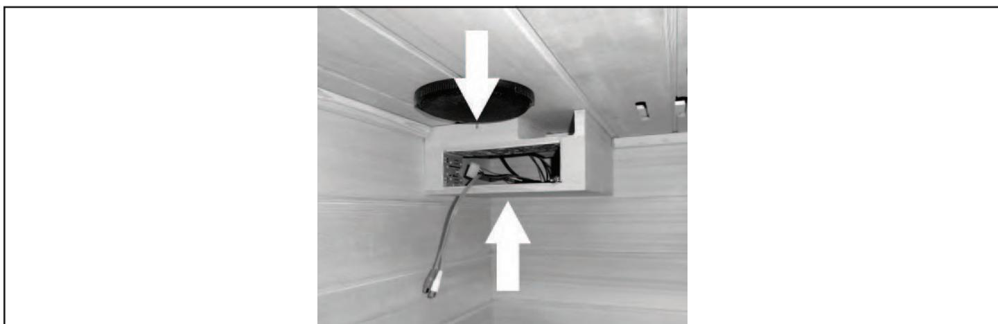
15. Plug the controller and antenna into the back of the AM/FM CD PLAYER. Slide and lock the AM/FM CD PLAYER into the STEREO SHELF.
