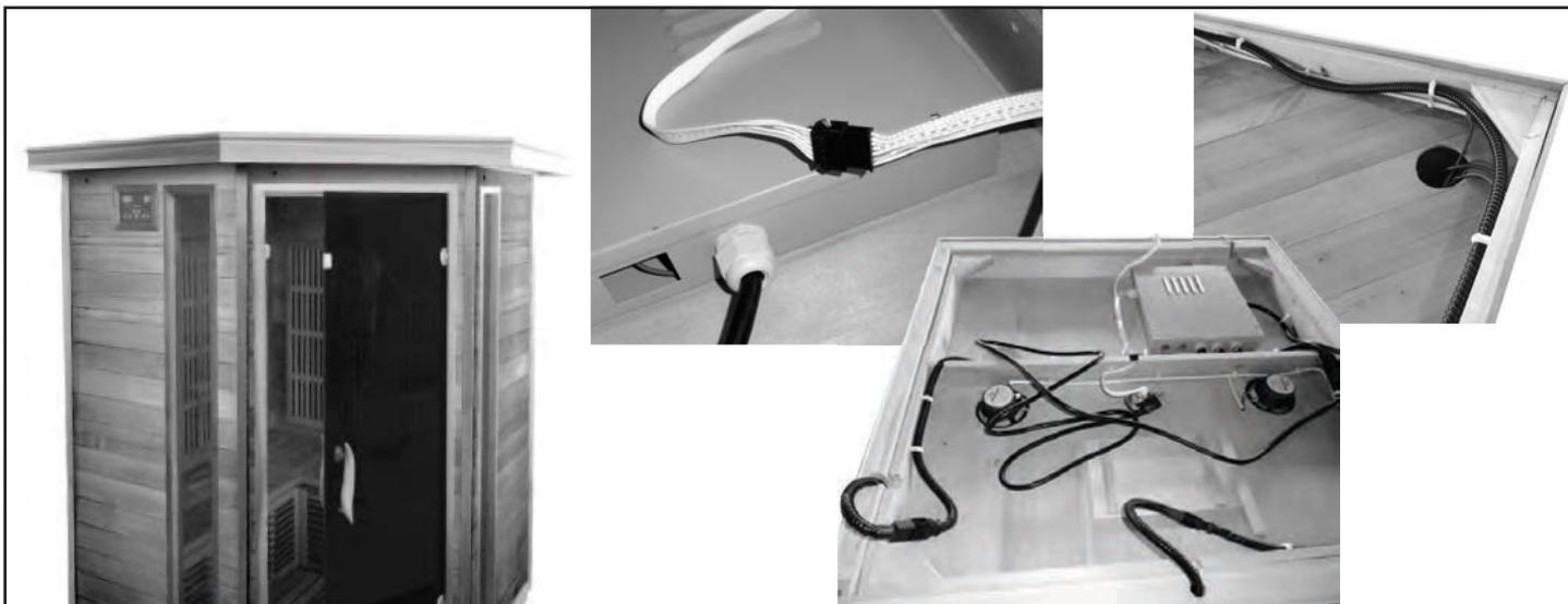
12. Feed the main power cable through hole in ROOF and plug securely into receptacle on back of POWER SUPPLY box . Secure the ROOF COVER with 3/4" SCREWS.
