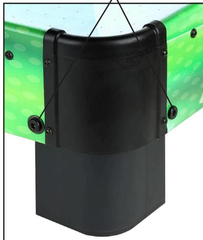
Legs to be black injection moulded ABS and should flush mount to table securely with 2 bolts, washers and nuts. Black EVA pads on bottom.
