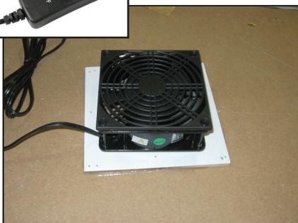
Securely mounted 5 blade axial fan AC120V 50/60 Hz 0.28A 24W 2P w/ new mounting board system going width of table.
