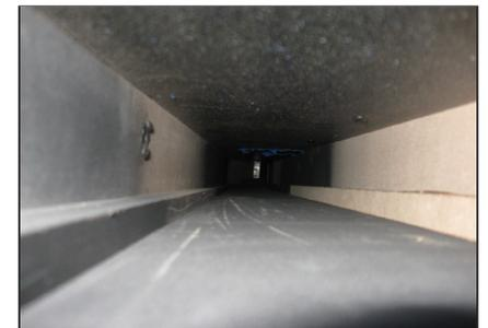
Ball return liners should be firmly glued in place with NO bubbles or wrinkles.
