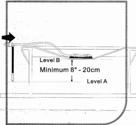
Place the drainer in the middle of your cover, and attach the siphon to the other side of the hose. Make sure that the tube of the siphon is lower than the drainer.
