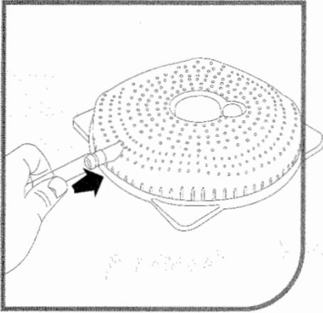
Plug the hose to the weighted head, and make sure that there are no knots.
