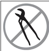
DO NOT USE TOOLS TO LOOSEN OR TIGHTEN TELESCOPING LEGS.
