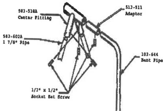
**STEP #3:** Plumb & level. Tighten all set screws using a short length of pipe on socket key to add leverage. Pour concrete and crown surface for drainage. Let stand 48 hours before removing braces, installing resilient surfacing and using equipment.
