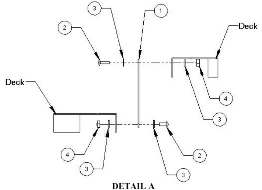
**5) Layout holes for Safety Enclosure/Barriers:** The top of the Safety Enclosures/Barriers should be 38" from the top of the surface of the deck to the top of the Safety Enclosures/Barriers. With help, hold the Safety Enclosures/Barriers up to the post that it will connect to and mark the hole with a dry erase marker. Drill these holes with the #7 drill bit. Repeat this step for the other side of the Safety Enclosures/Barriers. (See Detail A)
