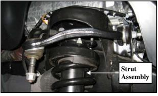
19. Install the lower strut bolt in the original position and torque to manufacturers specifications.
