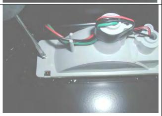
38. Fit lights using screws supplied in fitting kit, taking note of RH and LH light bodies, they are different and must be placed on the correct side of bull bar. Vent holes must be down,
