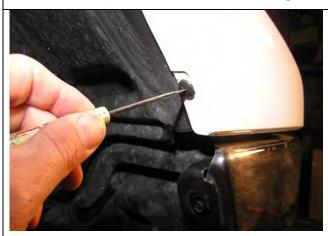
5. Remove upper fender liner retaining scrivets.
