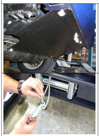
80. Fit stone tray using 4 x M8 bolts and washer sets at front and 2 x M8 bolts, washers and into fitted M8 cage nuts at two locations into existing sump guard front section as shown.
