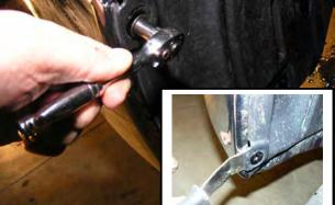
4. Remove all lower fender liner retaining screws to bumper.
