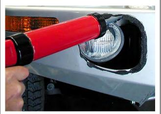
72. Note that the aperture moldings are handed (RH or LH), select correct hand for each wing aperture. Apply Sikaflex to recess in aperture molding flange or face of wing then fit molding aperture in wing.
