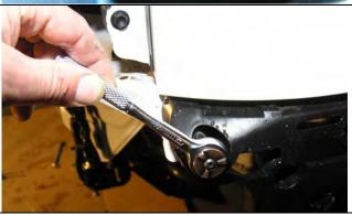
22. Remove bumper cover retaining brackets from the fenders.
