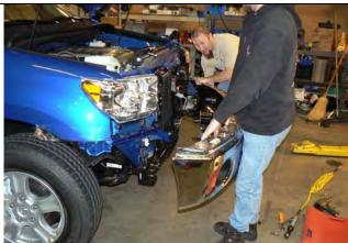
Remove crash bar and lower bumper assembly and set aside, retain flange nuts for reuse.
