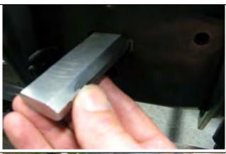
24. Insert clevis nut into rectangular hole in the inboard face of chassis, ensuring the threaded end is inserted first.
