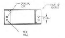
In some cases, the roller fair lead bracket must have a second set of holes drilled to line up with holes in winch bracket. If required, mark out as shown and using a 13.0 mm drill bit, drill two holes as shown in diagram.
