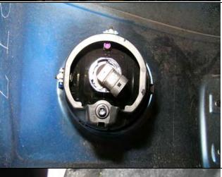
7. If OE fog lights and/or parking sensors fitted in bumper, undo electrical connections.
