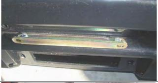
39. Secure the number plate bracket using M6 bolts, flat washers and flange nuts. Attach the longer side to the bullbar and the shorter side to the number plate.
