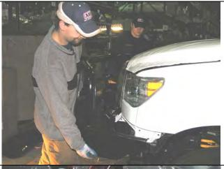
56. Using two people, three if winch fitted, position the bar assembly on the vehicle mounts.
