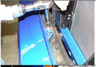
14. Remove screws located along top of cross member retaining upper bumper metal frame.
