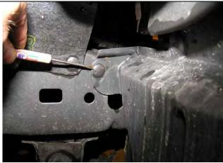
Prise out lower fender liner plastic push in plugs. Remove lower fender liner completely, they will not be reused.
