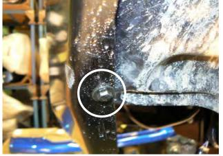
77. Then secure fender liner using M6 x 20 black bolts and 2 x black washers with flange nut.
