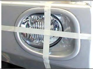
73. Use adhesive tape to secure plastic mold while Sikaflex cures.
