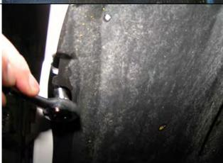
8. Remove bumper wing retaining screws in upper wheel arch area.
