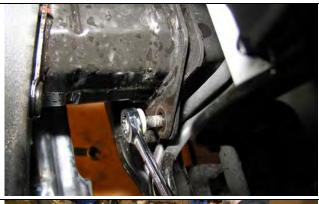
18. Undo crash bar mounts from chassis flange.
