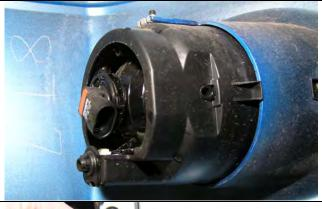
21. Remove OE fog lamps if fitted and are to be reused. The plastic surrounds are not to be reused.
