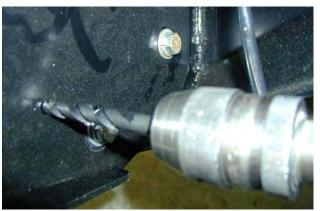
64. Using the M10 pilot hole in mount brackets, drill pinning hole through uprights of bull bar. Fit M10 SEMS bolt and flange nut, do up tight.
