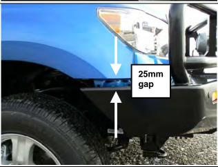
61. Adjust the bar height leaving approximately 25mm gap between top of wing to fender.
