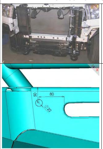
29. Centralise the brackets to vehicle and then check the outside measurement across mount brackets, it needs to be 930mm or less. Nip up the M10 flange nuts and tow hooks to better secure mount brackets to chassis.
