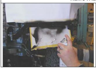
23. Mask up and spray paint the exposed metal trim area black satin, from the wheel arch right around to the inboard headlamp area as shown, both sides of the vehicle.
