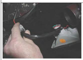
74. Wire up indicators and running lamps. Wire loom extensions are supplied in fitting kit.
