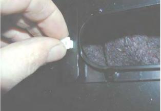
37. Insert nylon nuts into square holes in light brackets inside wing area.
