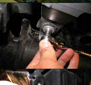
3. Remove lower bumper retaining screws.
