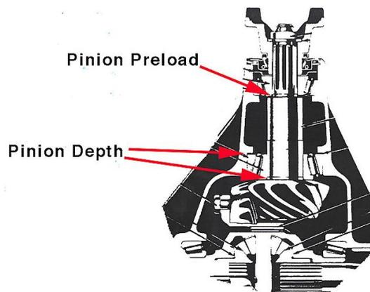
Pinion depth is controlled by shims. Shims may be located between the inner pinion bearing & pinion head or they may be between the inner Pinion bearing cone and carrier housing. In either case removing a shim will Move the pinion away from the center line of the ring gear while adding a shim will move it toward the centerline
