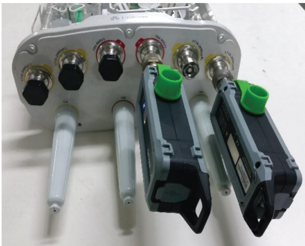
Equipment setup for measuring antenna isolation with two iVA-TMAs
