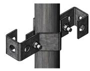
PIM-guard Round Member Cable Support Bracket 6 ports for stackable hangers (up to 3 per port). Install with torque wrench set at 5 to 7 ft-lb to meet carrier PIM requirements. For patents, see www. cs-pat.com
