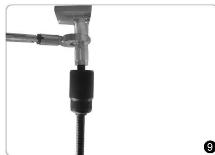
Tighten with torque wrench. Recommended torque is 25N·m.
