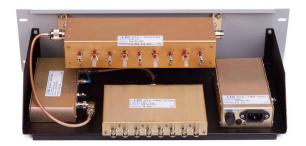
EMR Receiver Multicouplers allow several receivers to share a common antenna. These units include a preselector, amplifier, power supply and power divider which effectively amplifiy a filtered band of frequencies to individual receivers. The power divider provides a minium 20 dB of port-to-port isolation preventing signal mixing even at minimal channel separation.
