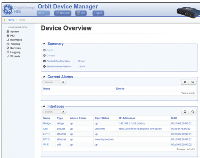
The Orbit Device Manager overview page provides critical information at-a-glance such as active alarms and high-level interface status.
