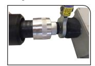
Torque the connector to 18 ft. lbs. using the TQ-114-F18 torque wrench and adjustable wrench.
