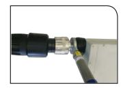
Torque the connector to 18 ft. lbs. using the TQ-114-F18 torque wrench.
