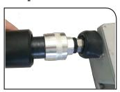
Connect the JMA 1-5/8" DF connector to the antenna port or device and hand tighten.
