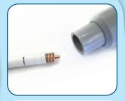
No coring of dielectric is necessary. Hold prepped cable end at a downward angle, tapping the cable while vacuuming.
