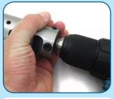
Attach prep/strip tool to drill. Be sure to use SP-12PL tool. Prepping cable on the spool is recommended for lengths under 6'.
