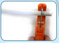
Straighten cable. Using RDCUTTER-S, apply even pressure while rotating tool around cable to cut off cable squarely.
