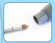
Hold prepped cable end at a downward angle, tapping the cable while vacuuming a second time.
