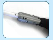
Actuate drill to remove jacket and expose the center conductor until the prep tool reaches the mark made on the jacket, and the final cut is in the valley.
