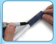
Slide blue marking guide over cable until it bottoms on the first dielectric ring. Mark cable with a line at end of marking
