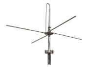
1-port omni ground plane antenna, 450–470 MHz, 360° HPBW, fixed electrical tilt. Bandwidth: 2% of frequency.
