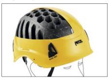
ALVEO helmets have an internal expanded polystyrene foam liner for reduced weight. Shock is absorbed by deformation of the expanded polystyrene liner. Weight: 350 g
