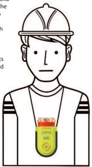
When the V-Watch Personal Voltage Detector is in use with a good working battery, it is always on, always ready to warn of potentially hazardous high voltage. The battery life is approximately six months of continuous use or two years in storage. When the job requiring the protection of the detector for the user is completed, the detector should be closed by pushing down on the top.
