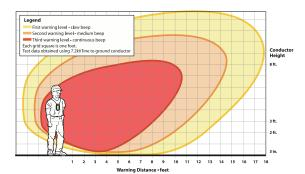
Conductors of different phases in close proximity will also reduce warning distances due to field cancellation effects.
