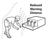
The V-Watch Personal Voltage Detector measures only the strength of the electric field. It cannot directly measure distance to the source of the electric field such as an energized conductor. The higher the voltage, the stronger the field and the greater the alarm
